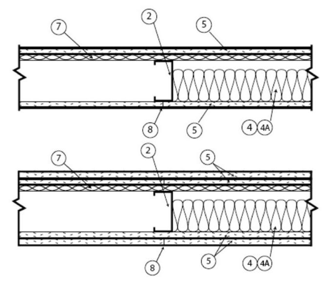
1. **Floor and Ceiling Runners** — (Not Shown) — Channel shaped, fabricated from min 25 MSG (0.018 in. min. bare metal thickness) corrosion-protected steel, min width to accommodate stud size, with min 1-1/4 in. long legs, attached to floor and ceiling with fasteners 24 in. OC max.
